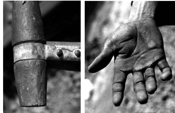
Figures 10 & 11 Due to the use of t-shaped grip of the shovel handle, their palms become very stiff and full of blisters
