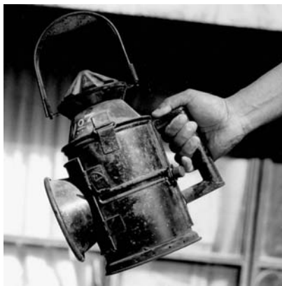
Figure 15 Small spaces between handle and the body lead to large number of burn injuries
